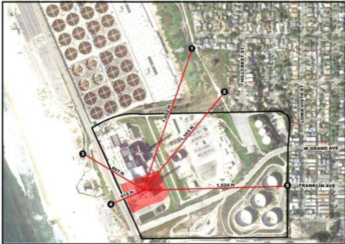
FIGURE 4.2.7-5. CONSTRUCTION SCENARIO 3 NOISE SOURCES AND SENSITIVE RECEPTORS
