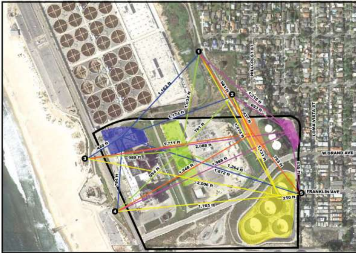
FIGURE 4.2.7-4. CONSTRUCTION SCENARIO 2 NOISE SOURCES AND SENSITIVE RECEPTORS
