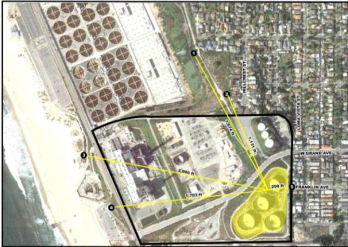
FIGURE 4.2.7-3. CONSTRUCTION SCENARIO 1 NOISE SOURCES AND SENSITIVE RECEPTORS
