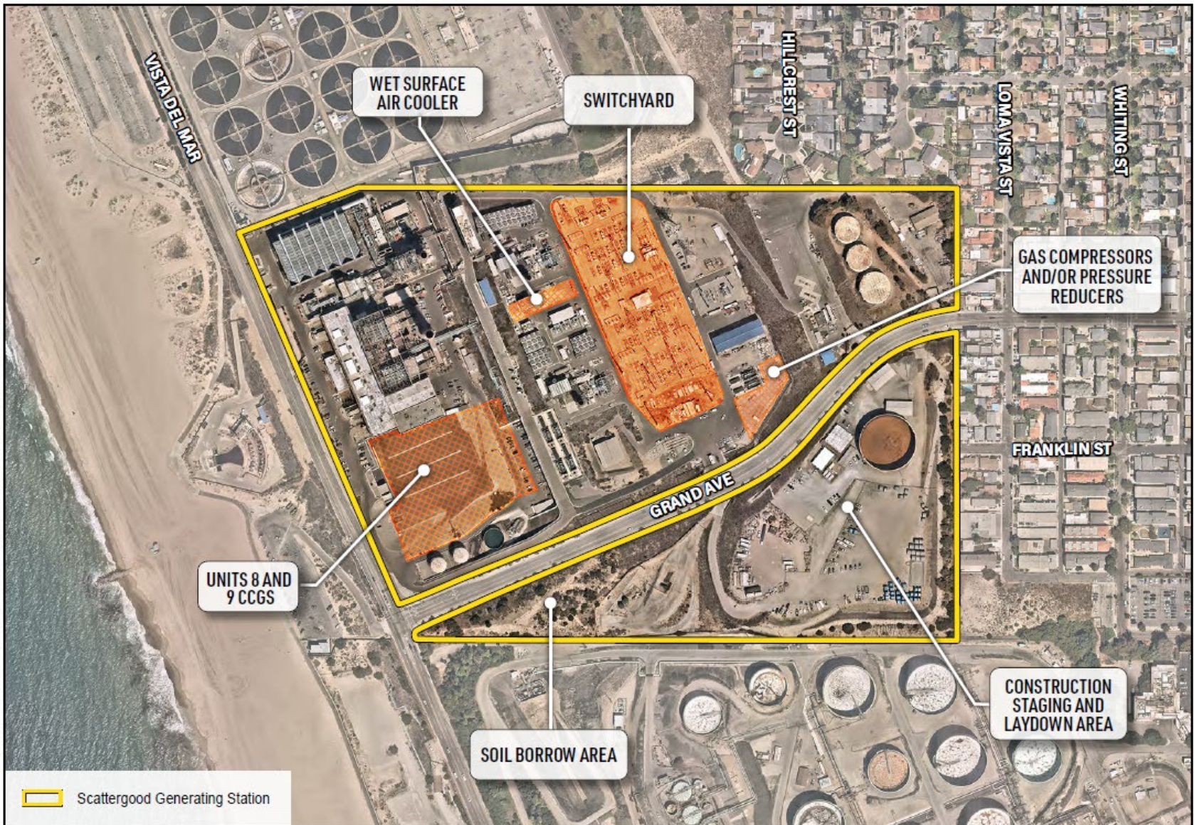
SCATTERGOOD GENERATING STATION UNITS 1 AND 2 GREEN HYDROGEN-READY MODERNIZATION PROJECT Proposed Project Components
