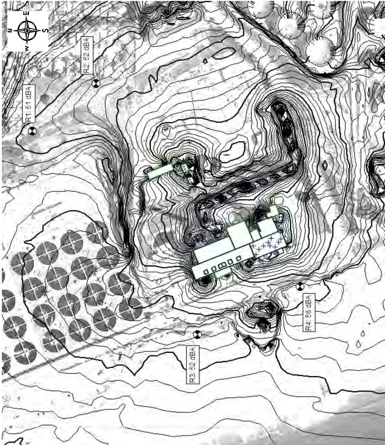
Figure 4: Noise Propagation from Scattergood Generating Station
