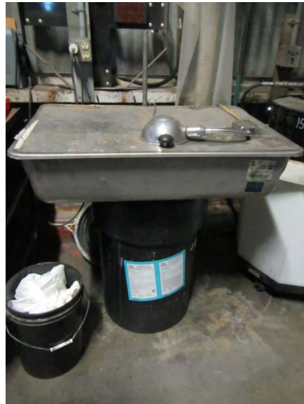
Photograph 20 – Photograph showing one of two parts washers in the auto service building.
