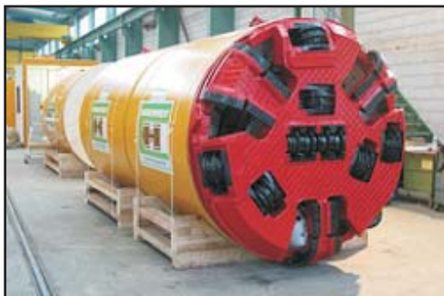
Microtunnel Boring Machine
